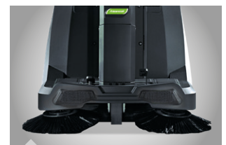
Working width without side brushes 580 mm
