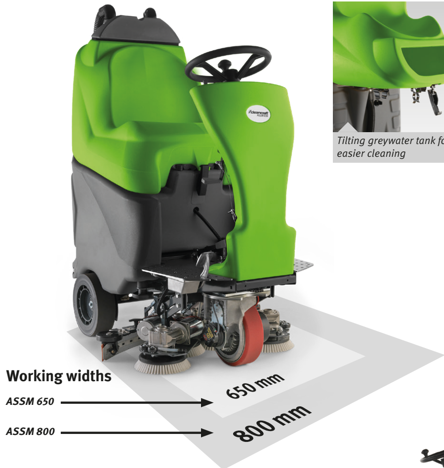
Four small disk brushes, with a vacuum rail directly behind them allow for a short design and a very tight turning circle
