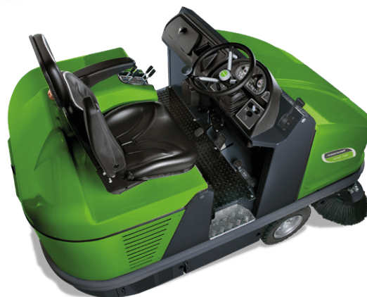
Hydraulic emptying of waste container up to a height of 1.5 m
