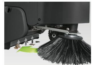
Side brushes with electrical dust extraction
