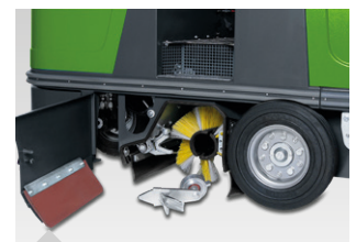
Main sweeping roller and side brushes can be replaced without tools
