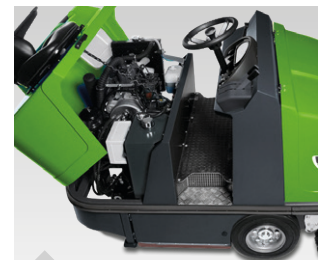
One focus in the design phase was convenient access, thus ensuring that regular maintenance work can be performed quickly and easily
