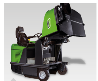
Hydraulic emptying of waste container up to a height of 1.5 m
