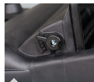
HKM 800: Easy height adjustment of sweeping rollers without tools
