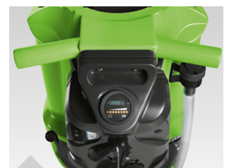
Mechanical operation of brush and vacuum rail via levers
