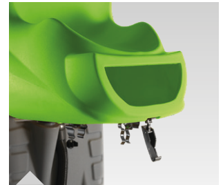
Tilting greywater tank for easier cleaning
