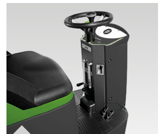
Mechanical operation of brushes and vacuum rail via levers
