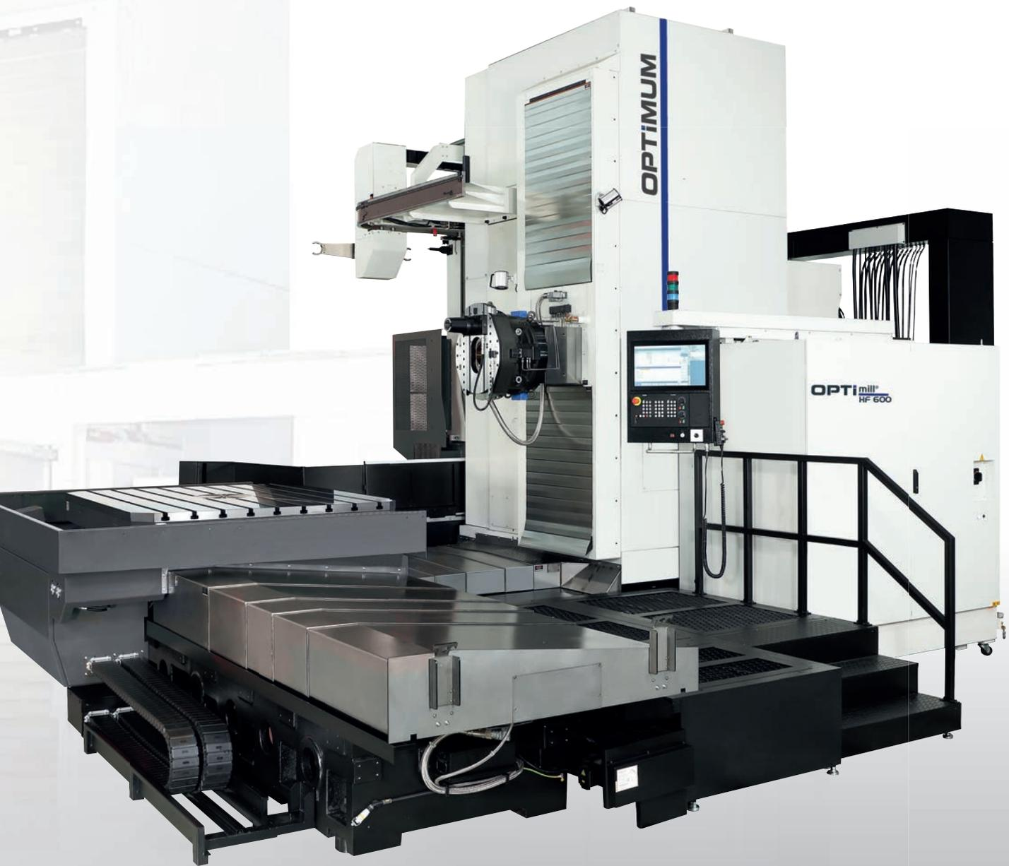
Horizontal drilling and milling centre HF 400
