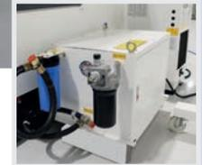
Fig. Filter unit internal 20 bar
