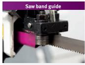
> Ball-bearing borne; for an excellent band run and thus optimal cutting
