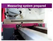
> Prepared for measuring system installation on the X, Z and ZO axis
