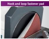
Good grinding wheel adhesion, easy replacement
