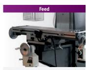
Table feed on X- and Y-axis with speed adjustment
