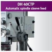
> Drilling depth stop adjustable within range of 0-120 mm. The feed is automatically switched off after reaching the preset drilling depth and turned back to its original position by the spring force of the return spring
