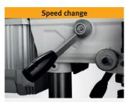
> The infinitely variable V-belt drive is used to position the V-belt to the desired V-belt diameter with the hand lever while the drilling spindle is rotating. This causes the speed to change
