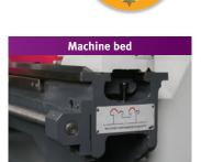
> Grey cast iron prism bed with strong ribbing, aged for at least six months, induction tempered and precision
