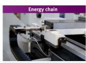
> for routing that is easy on the cable and hose material
