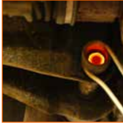
For heating and loosening jammed and corroded parts
