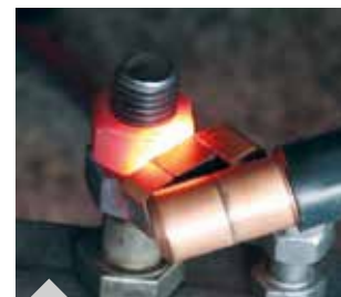
Heating a nut with the angled focusing coil
