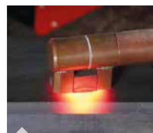
Heating a component with the straight focusing coil
