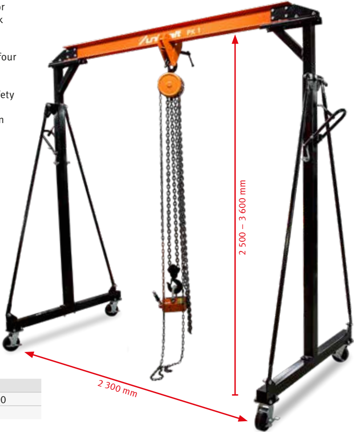
Safe and easy height adjustment in unloaded state via levers and two safety bolts per support carrier
